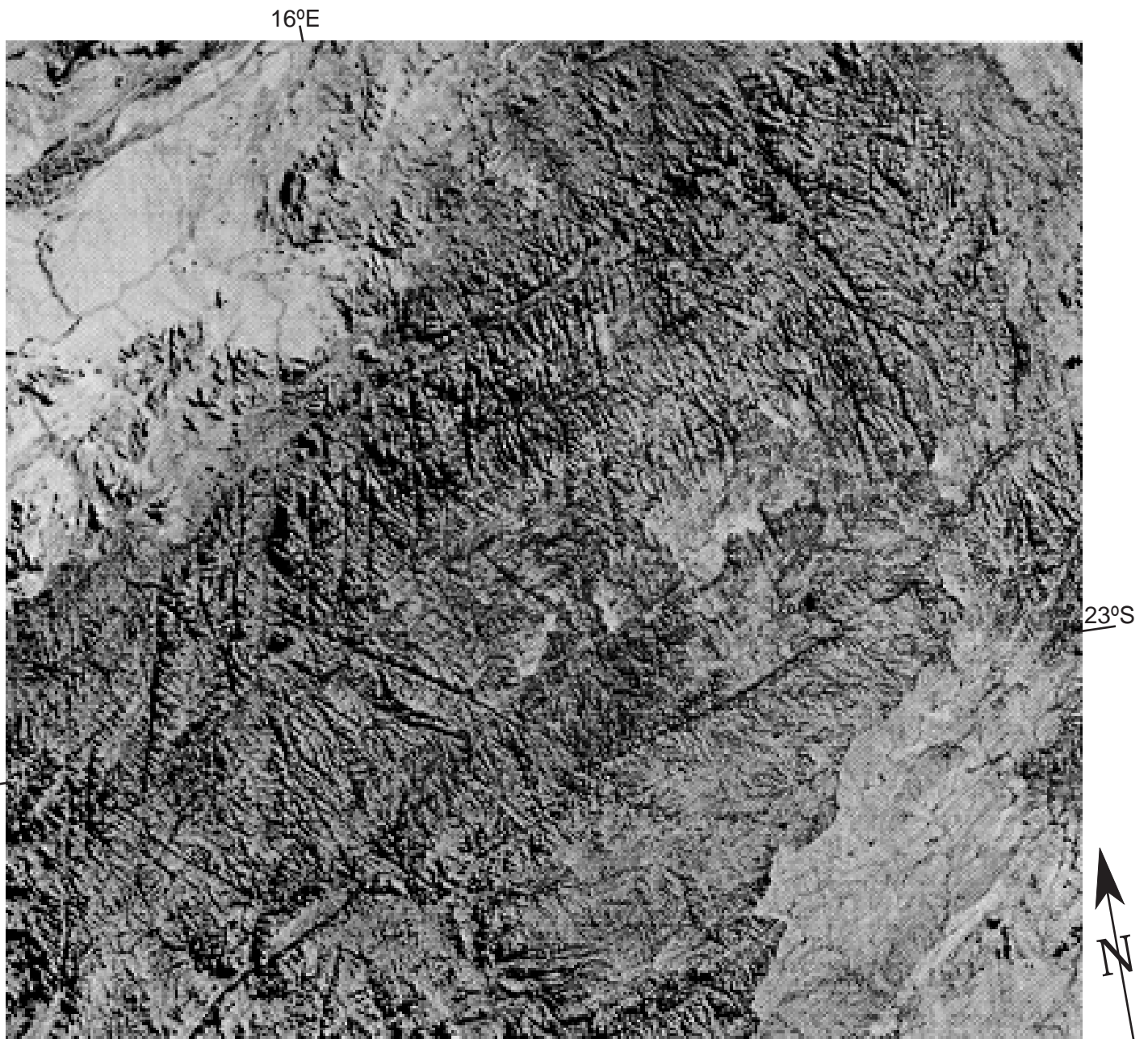
Figure 6. Landsat image of a portion of the African shield in Namibia showing 3 principal fracture sets of different strike directions. From Short, et al, 1976, p. 384. Landsat and radar images of outcropping basement worldwide show similar fracture sets, leading us to believe that all continental crust is equally fractured. In outcrop these "fractures" are, in reality, high metamorphic grade shear zones. Would a later orogeny in this area create new shear zones or simply reactivate the ones shown?
