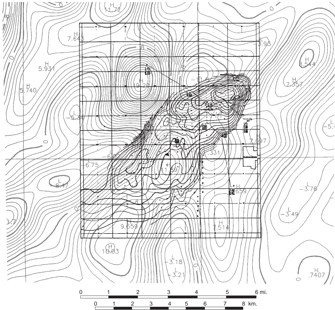
FIGURE 12. Cunningham Field, Pratt and Kingman Counties. Close correlation of the underlying basement shear zone with the asymmetric anticline indicates a probable reverse fault here, as in other similar fields in Kansas and Oklahoma. Black contours are on top of the Lansing formation; gray contours are residual magnetics. Structure is from Skelly Oil Company, Geology Dept., 1956.
